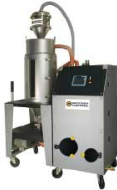
Portable Drying and Conveying 25 to 300 lbs/hr
